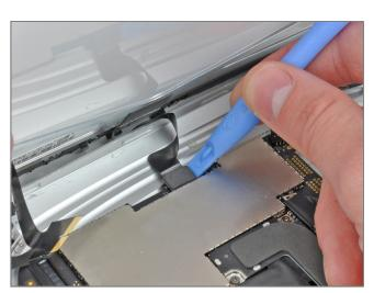
Use an iPod opening tool to remove the ambient light sensor connector from its socket by gently prying upward.
